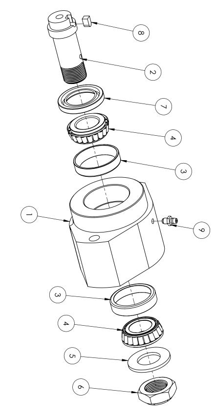
NOTE: WHEN REPAIRING/REBUILDING BEARING BLOCK, LOCK NUT (2902961) MUST BE TORQUED TO 50LB-FT. ROTATE SHAFT BY HAND TO ENSURE NO END PLAY IN SHAFT, SHAFT SHOULD NOT BE OVERTIGHTENED.
