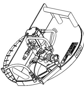
MAXIMUM CUTTING DEPTH HYDRAULIC CONNECTIONS **BLADE FLANGE** SAW WEIGHT **BLADE RPM** Flush Cut, 6 on 3.50" 5/16-18 x 82° CS 40lbs, No Blade, No Cover Parker No Spill 1/2" 2250 rpm @ 10 gpm 2500psi - 10 gpm 10.00"
