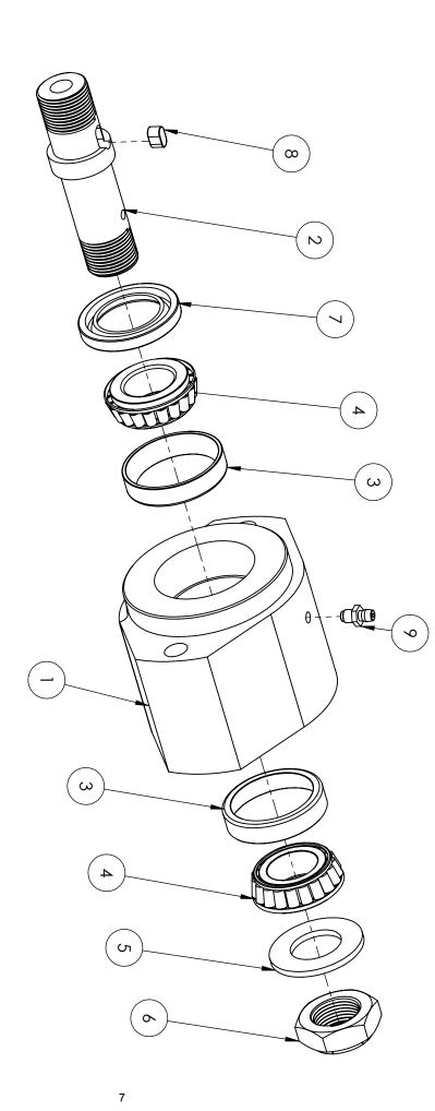
NOTE: WHEN REPAIRING/REBUILDING BEARING BLOCK, LOCK NUT (2902961) MUST BE TORQUED TO 50LB-FT. ROTATE SHAFT BY HAND TO ENSURE NO END PLAY IN SHAFT, SHAFT SHOULD NOT BE OVERTIGHTENED. WHEN REPAIRING/REBUILDING BEARING BLOCK, GREASE ADEQUATELY USIING NLGI No.2 GREASE. BEARING BLOCK GREASE CAPACITY IS 1.5oz.
