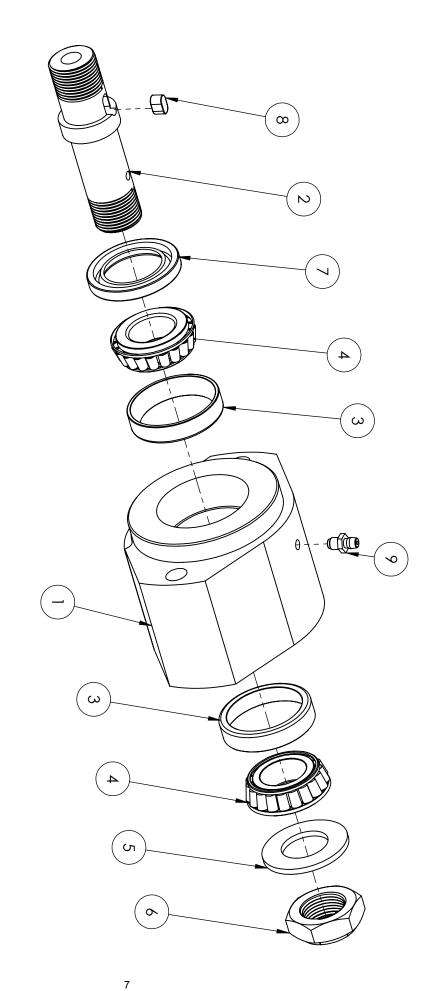
NOTE: WHEN REPAIRING/REBUILDING BEARING BLOCK, LOCK NUT (2902961) MUST BE TORQUED TO 50LB-FT. ROTATE SHAFT BY HAND TO ENSURE NO END PLAY IN SHAFT, SHAFT SHOULD NOT BE OVERTIGHTENED.
