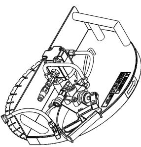
HYDRAULIC RECOMMENDATION2500psi - 8 gpmBLADE RPM2075 rpm @ 8 gpmHYDRAULIC CONNECTIONSParker No Spill 1/2"MAXIMUM CUTTING DEPTH10.00"SAW WEIGHT40lbs, No Blade, No CoverBLADE FLANGEFlush Cut, 6 on 3.50" 5/16-18 x 82° CS
